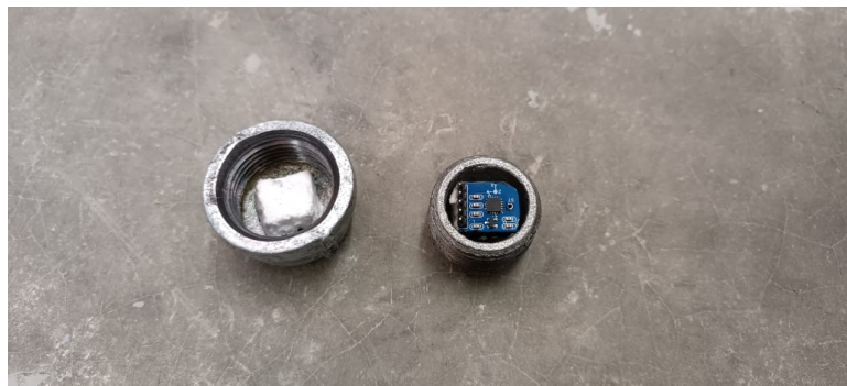
Figura 3: ADXL335 accelerometers housed inside the steel capsule.
